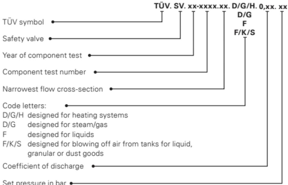
We check the safety valves for pressure resistance and tightness, adjust the requested set pressure and seal them. The identification on the type plate or on the spring bonnet of the valve is applied using a permanent marking system. The type plate is additionally marked with identification codes and technical data in compliance with DIN EN ISO 4126-1.
